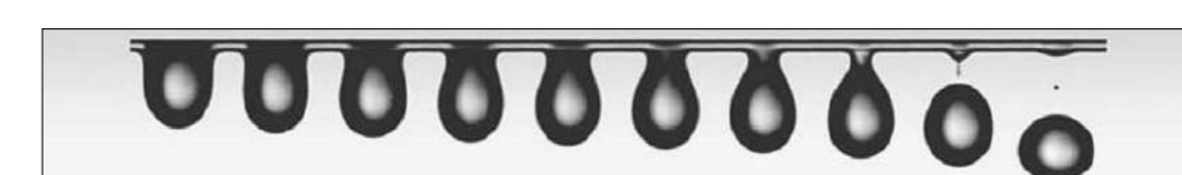
Fig. 2. Set of pictures showing a drop of silicon oil falling off a fiber of radius b = 350 \mu\text{m} . The volume of the drop is just above Q_{M,0} so that gravity dominates the capillary force: the drop falls (interval between two successive pictures: 1 ms).
